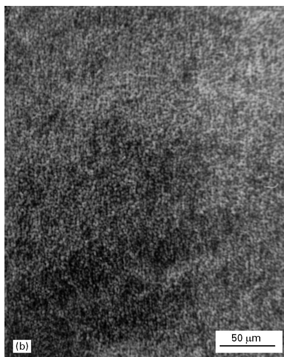
Figure 11 Surface of the sulphide scales formed on cobalt at T > 900 K and sulphur pressures (a) lower, and (b) higher than the dissociation pressure of \text{CoS}_2 .
