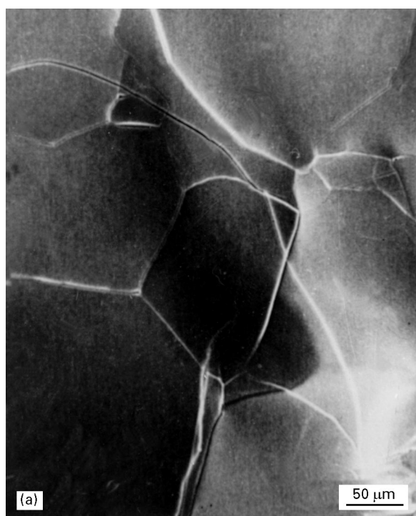
Figure 11 Surface of the sulphide scales formed on cobalt at T > 900 K and sulphur pressures (a) lower, and (b) higher than the dissociation pressure of \text{CoS}_2 .
